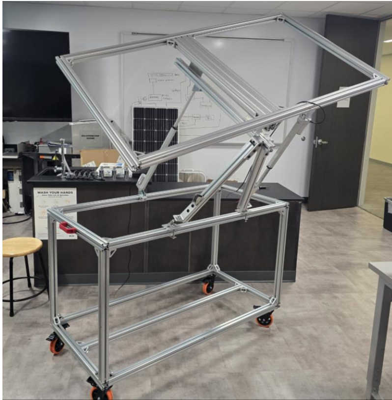
Figure 4. Team-A solar tracking charging cart
